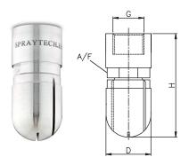
EB series self rotating nozzles are designed as a small dimensions and opening and perform inside cleaning which is required. Typically used for cleaning like kegs, small container where the requirement is for cleaning. Diameter of nozzle is (25mm) These nozzles are available in all grade of stainless steel.
